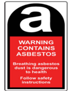
Figure 2 - Another type of asbestos label
